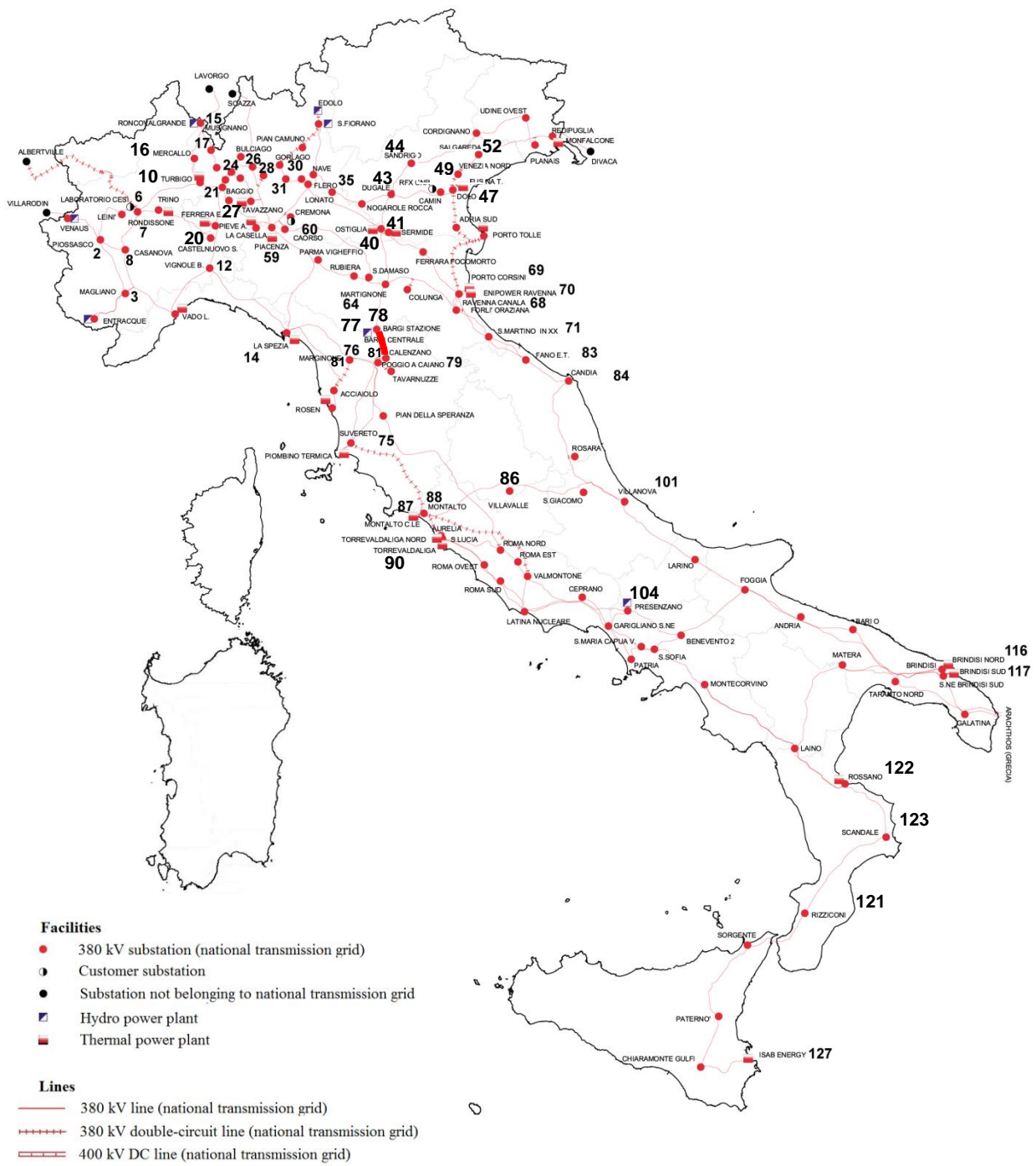
Figure 1. The 380 kV Italian power transmission network [52]
