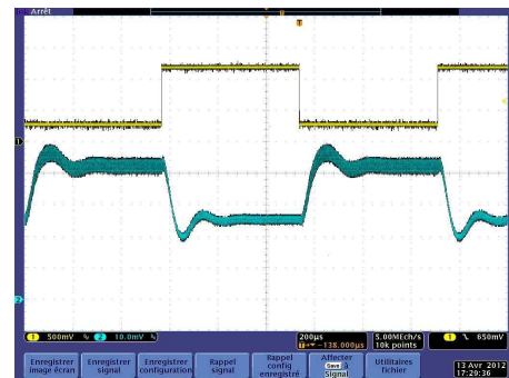
Fig. 15. Experimental result for another LED with V_0 = 11V and R_L = 3\Omega .
