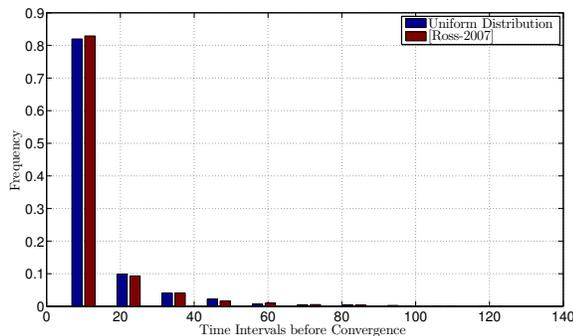
Fig. 3. Histogram of the convergence time to a SE in the game  $\widehat{\mathcal{G}} = (\mathcal{K}, \{\mathcal{A}_k\}_{k \in \mathcal{K}}, \{f_k\}_{k \in \mathcal{K}})$  using the algorithm (Alg. 1). Here,  $\text{SNR} = \frac{p_{k,\max}}{\sigma_k^2} = 10$  dBs,  $(\Gamma_1, \Gamma_2) = (1.5, 1.5)$  bps and  $N_1 = N_2 = 32$  power levels.
