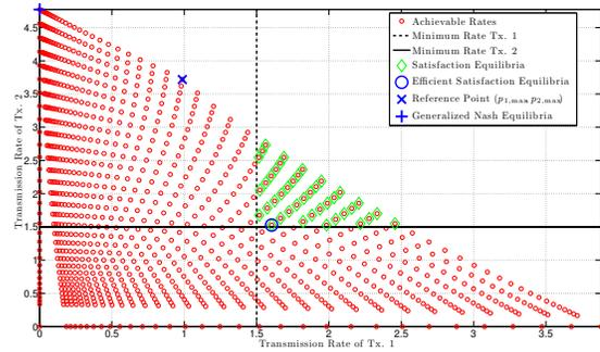
Fig. 2. Achievable (Shannon) transmission rates  $(u_1(p_1, p_2), u_2(p_1, p_2))$ , for all  $(p_1, p_2) \in \mathcal{A}_1 \times \mathcal{A}_2$ , with  $\text{SNR} = \frac{p_{k,\max}}{\sigma_k^2} = 10$  dBs,  $(\Gamma_1, \Gamma_2) = (1.5, 1.5)$  bps and  $N_1 = N_2 = 32^2$  power levels.
