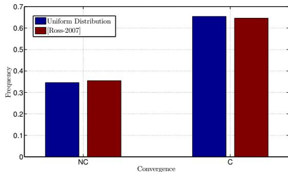
Fig. 4. Histogram of the event of convergence or non-convergence of the learning algorithm (Alg. 1) in the game  $\widehat{\mathcal{G}} = (\mathcal{K}, \{\mathcal{A}_k\}_{k \in \mathcal{K}}, \{f_k\}_{k \in \mathcal{K}})$ . Here,  $\text{SNR} = \frac{p_{k,\max}}{\sigma_k^2} = 10$  dBs,  $(\Gamma_1, \Gamma_2) = (1.5, 1.5)$  bps and  $N_1 = N_2 = 32$  power levels.
