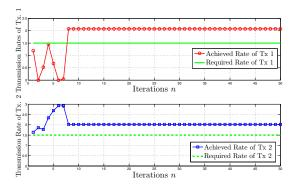
Fig. 5. Instantaneous achieved rates of transmitter 1 (red) and 2 (blue).Here, SNR =  $\frac{p_{k,\max}}{\sigma_k^2}$  = 10 dBs,  $(\Gamma_1,\Gamma_2)$  = (1.5,1.5) bps and  $N_1=N_2=32$  power levels.
