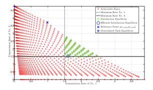
Fig. 2. Achievable (Shannon) transmission rates  $(u_1(p_1,p_2),u_2(p_1,p_2))$ , for all  $(p_1,p_2)\in \mathcal{A}_1\times\mathcal{A}_2$ , with SNR =  $\frac{p_{k,\max}}{\sigma_k^2}=10$  dBs,  $(\Gamma_1,\Gamma_2)=(1.5,1.5)$  bps and  $N_1=N_2=32$  power levels.
