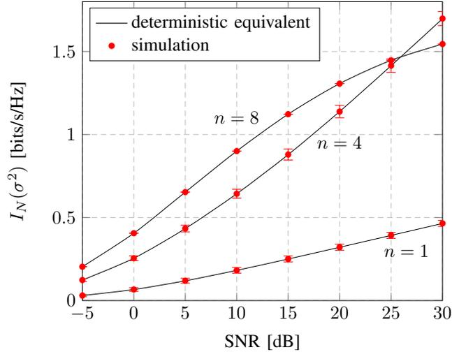
Fig. 2. Mutual information  $I_N(\sigma^2)$  versus SNR for different numbers of transmit signatures  $n$ ,  $N = 16$ ,  $N_i = 8$ ,  $\mathbf{P}_i = \mathbf{I}_n$ ,  $\alpha = 0.5$ . Error bars represent one standard deviation on each side.
