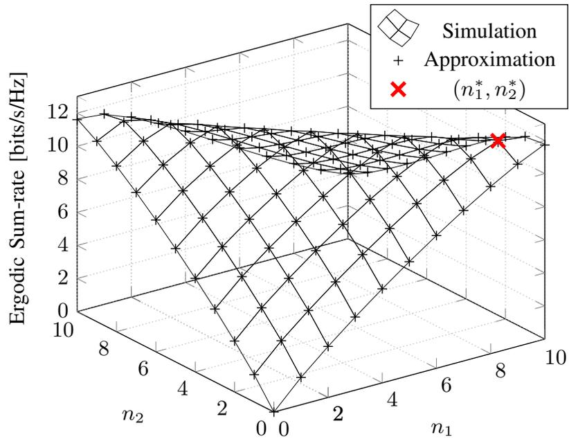
Fig. 8. Sum-rate versus number of transmitted data-streams  $(n_1, n_2)$  for SNR = 40 dB and all other parameters as provided in Table II. Solid lines correspond to simulation results, markers to the deterministic approximation by Theorem 4. As co-channel interference is dominant there is a clear gain of limiting the number of transmitted streams.
