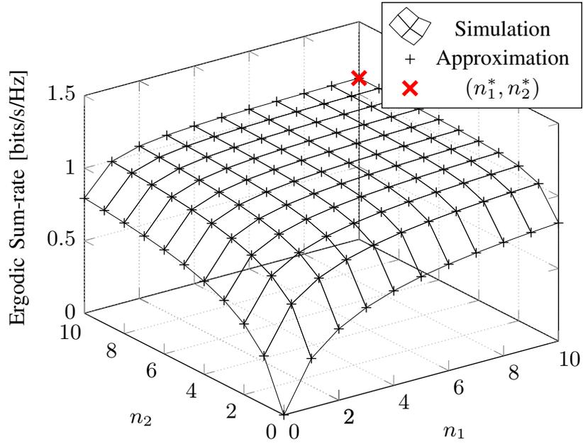
Fig. 7. Sum-rate versus number of transmitted data-streams  $(n_1, n_2)$  for SNR = 0 dB and all other parameters as provided in Table II. Solid lines correspond to simulation results, markers to the deterministic approximation by Theorem 4. As expected, both transmitters should send the maximum number of independent streams.
