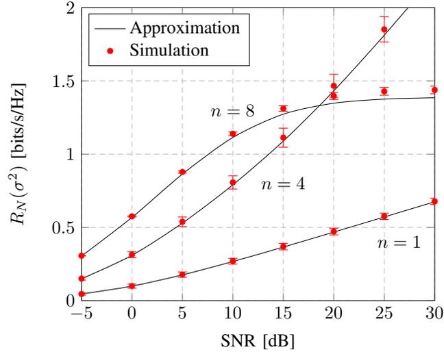
Fig. 3. Sum rate  $R_N(\sigma^2)$  at the output of the MMSE decoder for user 2 versus SNR for different numbers of transmit signatures  $n$ ,  $N = 16$ ,  $N_i = 8$ ,  $\mathbf{P}_i = \mathbf{I}_n$ ,  $\alpha = 0.5$ . Error bars represent one standard deviation on each side.
