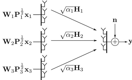
Fig. 4. MIMO MAC from three transmitters ( $k = 1, 2, 3$ ) with  $N_k$  antennas to a receiver with  $N$  antennas. Each transmitter sends  $n_k$  streams with precoding matrix  $\mathbf{W}_k$  and power allocation  $\mathbf{P}_k$  over the channel  $\sqrt{\alpha_k} \mathbf{H}_k$ .
