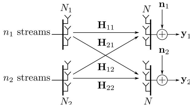
Fig. 6. Interference channel from two transmitters with  $N_k$  ( $k = 1, 2$ ) antennas, respectively, to two receivers with  $N$  antennas each. Each transmitter sends  $n_k$  independent data streams to its respective receiver.
