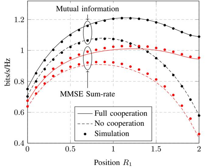
Fig. 2.  $I_c$ ,  $I_{\text{nc}}$ ,  $R_c^{\text{MMSE}}$ , and  $R_{\text{nc}}^{\text{MMSE}}$  and their asymptotic approximations by Propositions 3, 4, 5, and 6 versus  $R_1$ . Markers correspond to simulation results, solid lines to the asymptotic approximations.
