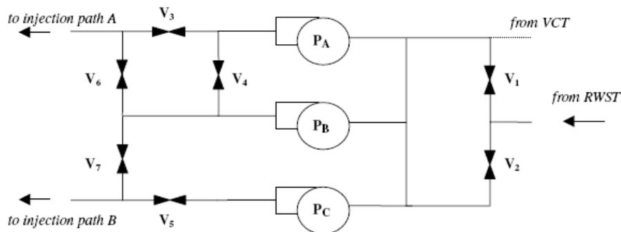
Figure 1: The simplified HPIS system (RWST = radioactive waste storage tank)<sup>9</sup>
