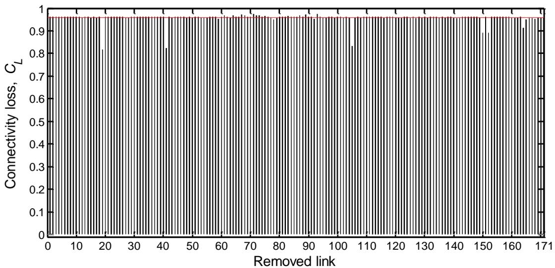
Figure 9. The connectivity loss,  $C_L$ , resulting from the initial attack on line 107 followed by the operator intervention of opening a line (abscissa). Horizontal line  $C_L = 0.96$  represents the reference connectivity loss, i.e. obtained without any further intervention after the attack
