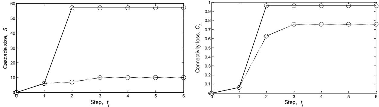
Figure 10. The cascade evolution in terms of cascade size,  $S$ , and connectivity loss,  $C_L$ , after the failure of line 107 and with no intervention at  $t = 1$  (solid lines) or optimal operator intervention at  $t = 1$  (dotted lines)
