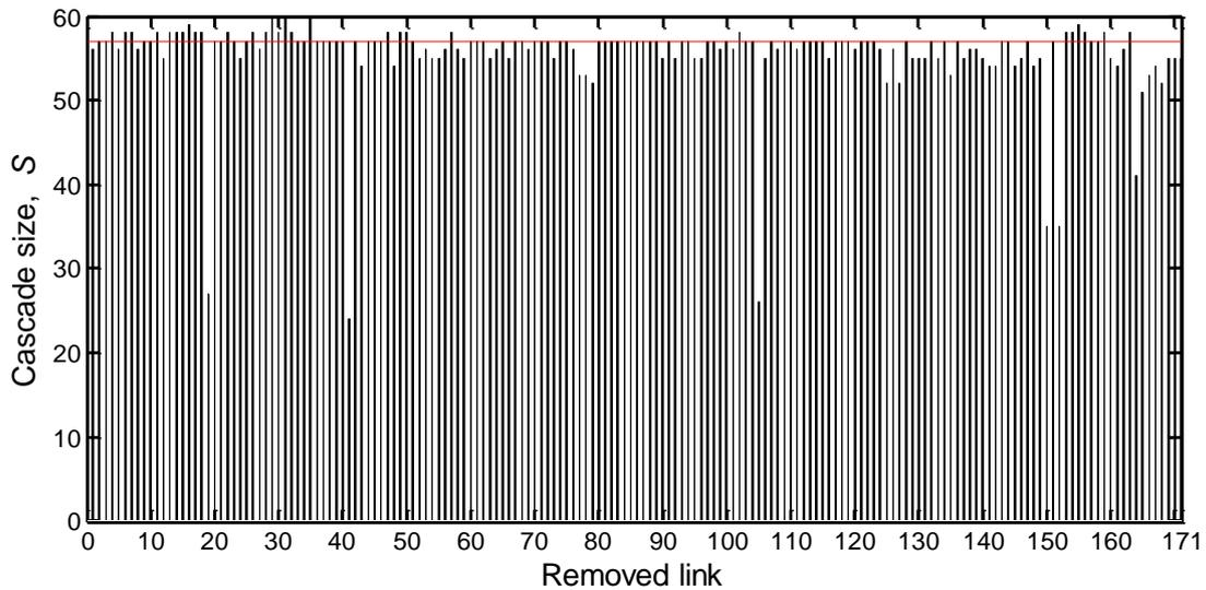
Figure 8. The cascade size,  $S$ , resulting from the initial attack on the line 107 followed by the operator intervention of opening a line (abscissa). Horizontal line  $S = 57$  represents the reference cascade size, i.e. obtained without any further intervention after the attack
