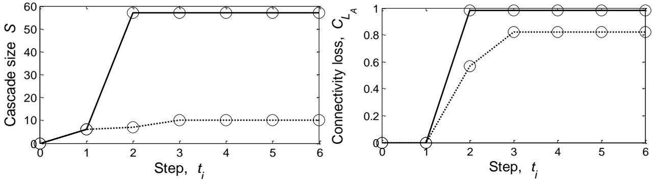
Figure 12. The cascade evolution in terms of cascade size,  $S$ , and local-area connectivity loss,  $C_{L_A}$ , after the failure of line 107 and with no intervention at  $t=1$  (solid lines) or optimal operator intervention at  $t=1$  (dotted lines)
