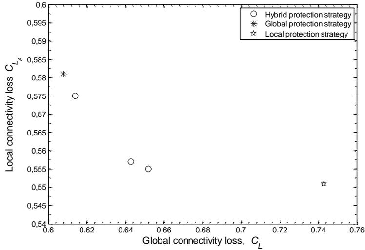
Figure 13. The Pareto frontier identified at  $t = 1$  after the multiple-line switching optimal operator intervention
