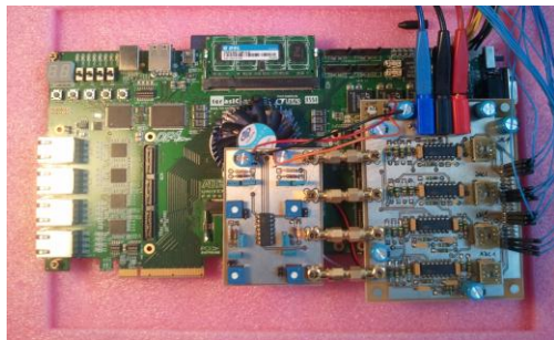
Figure 7. Experimental Set-up showing a digital FPGA development board associated with the analog front end used to emulate a MEMS resonant sensor
