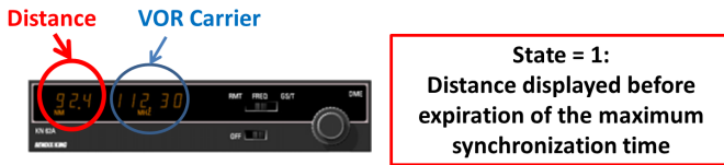
Fig. 10. Displayed information by the synchronized DME interrogator.
