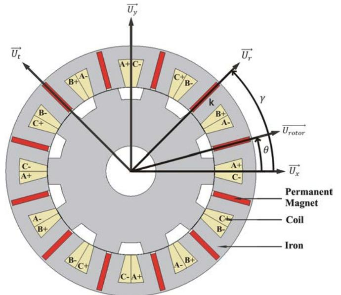
Fig. 2. 12/10 Flux Switching Permanent Magnet Machine
