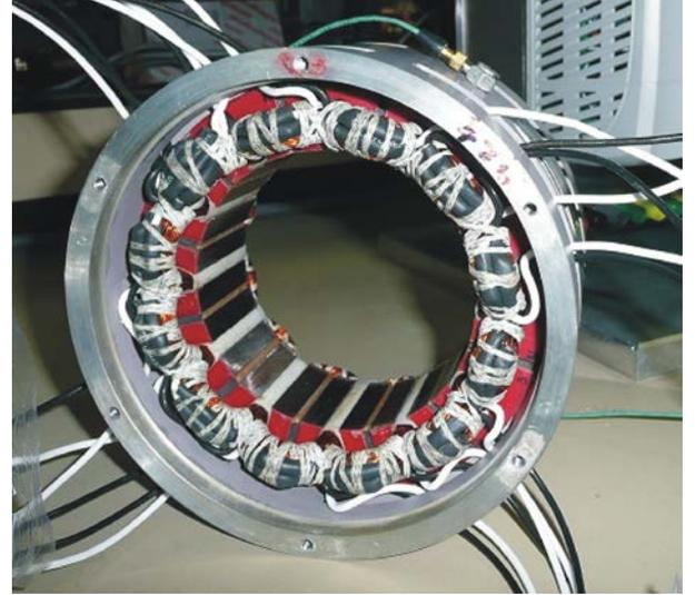
Fig. 9. FSPM stator and accelerometer
