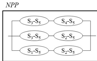
*Figure 11: Logic connections between the interconnected systems  $S_i$ ,  $i=1, \dots, 5$ , to the nuclear power plant (NPP).  $S_1$ : internal power system,  $S_2$ : internal water system,  $S_3$ : external power system,  $S_4$ : external water system,  $S_5$ : road transportation.*
