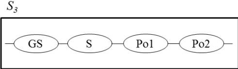
Figure 7: Logic connections between the components of the external power system,  $S_3$ . GS: Generation Station, S: Substation, Po: Pole
