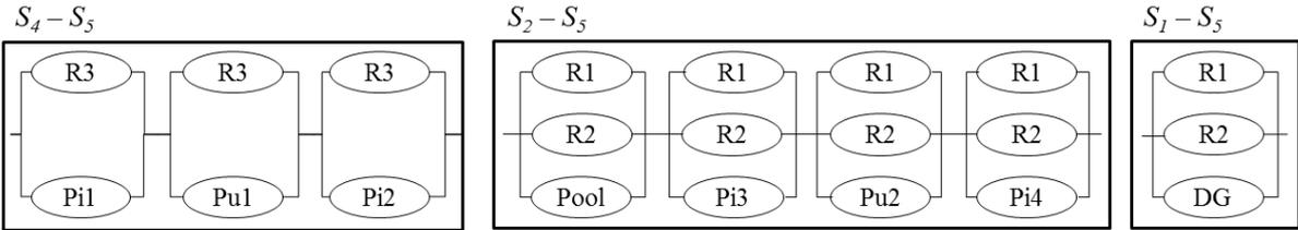
Figure 9: Logic connections between the components of the external water system,  $S_4$ , internal water system,  $S_2$ , internal power system,  $S_1$ , and those of the road transportation,  $S_5$ . GS: Generation Station, S: Substation, Po: Pole, Pi: Pipe, Pu: Pump, DG: Diesel Generator, R: Road access.
