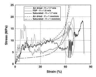
**Fig. 11** Mechanical behaviour of poplar at different moisture contents for quasi-static and impact tests. The resonance of the moving mass is highlighted by a *circle* at the end of the compression plateau
