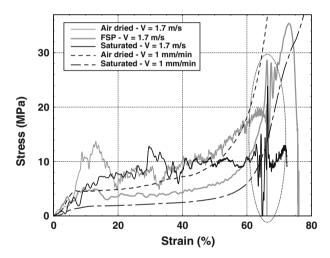
**Fig. 10** Mechanical behaviour of spruce at different moisture contents for quasi-static and impact tests. The resonance of the moving mass is highlighted by a *circle* at the end of the compression plateau
