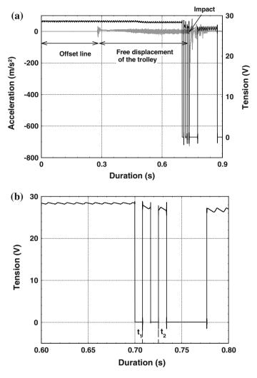
Fig. 3 Original data obtained during a test. Tension (*black curves*) and acceleration (*grey curve*) recorded during a test (a), with details of the photosensor signal used to determine the two instants  $t_1$  and  $t_2$  (b)
