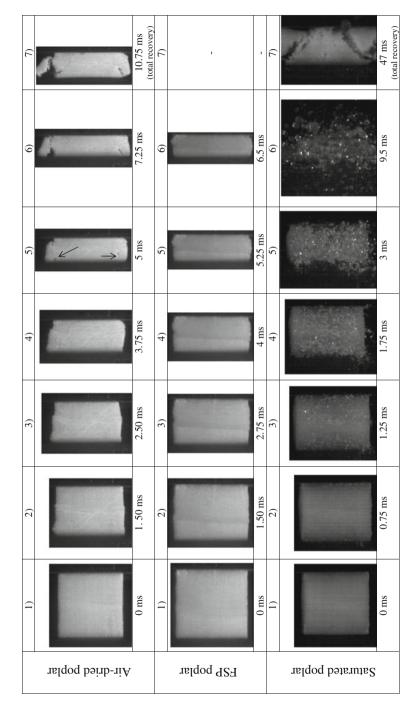
Fig. 8 Deformation of air-dried, FSP and saturated poplar wood during dynamic compression
