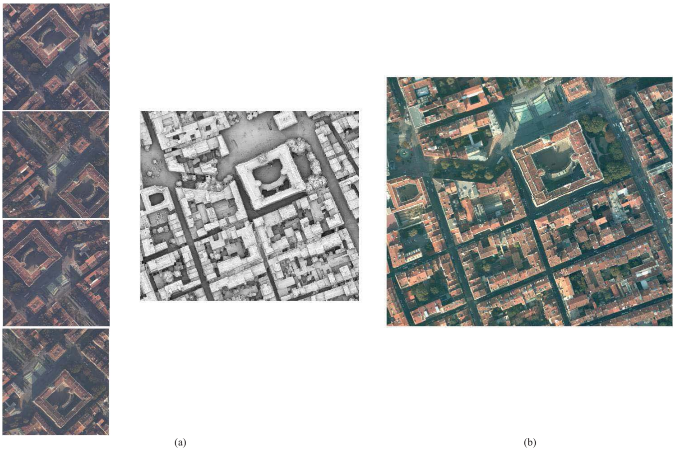
Fig. 4. Sample data acquired over the city of Marseille in 2004. (a) Set of four images from two neighbor flight strips in which the same building is visible. There are high-resolution RGB images in a conique perspective. The DSM obtained by correlation from the multiview images. (b) Resulting orthophotograph of the same area.
