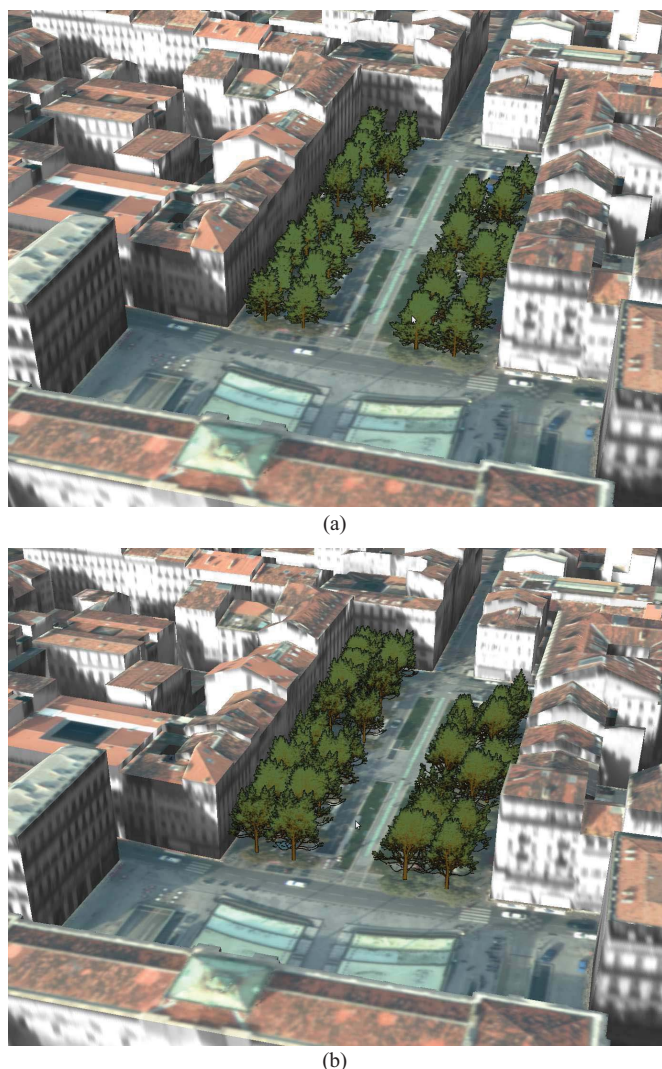
Fig. 10. Three-dimensional city model including functional vegetation models. (a) Trees are represented by billboards obtained from screenshots of the functional tree models exploiting tree height and crown areas estimated for each tree crown. (b) 3-D city model presenting the time evolution of the vegetation cover including five-year older vegetation models for the reconstructed area.
