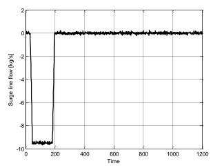
Figure 11 Evolution of the surge line flow rate
