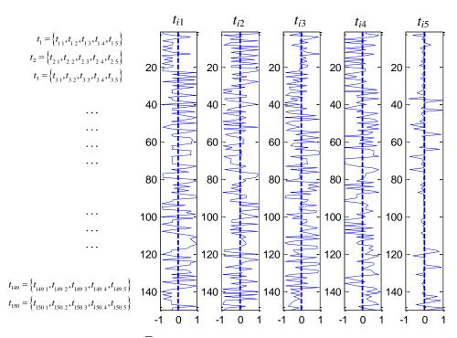
Figure 7 Representation of matrix T. Columns correspond to the values of the first 5 eigenvectors of  $L_{sym}$  of the raw data matrix of Figure 5
