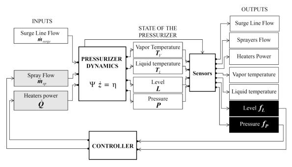
Figure 10 Inputs, state, controller outputs (gray), controller inputs (black) and sensors outputs of the SIMULINK model of the pressurizer
