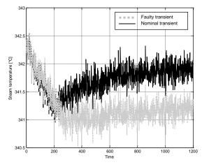
Figure 17 Evolution of the steam temperature for a nominal transient and the faulty transient
