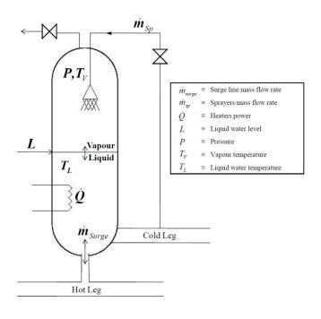
Figure 9 Simplified model of a pressurizer
