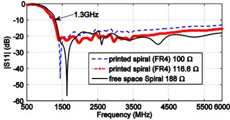
Fig. 2. Calculated reflection coefficient (S11) of elementary spiral
