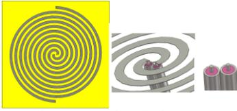
Fig. 1. Elementary spiral antenna and its feeding system
