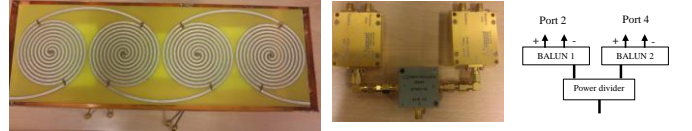
Fig. 5. The antenna array and the used feeding circuit composed of two pulse lab PSPL BALUN and a power divider in the middle of the photography.
