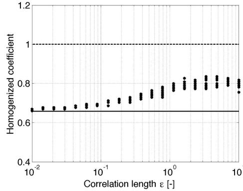
Figure 9. Convergence of the Arlequin estimate  $\underline{K}_N^\epsilon$  as a function of the correlation length  $\epsilon = \ell_c/L$ , for different ensembles of  $N = 10^3$  realizations of the random medium. The dashed line indicates the value of the arithmetic average  $E[\mathbf{k}_\epsilon]$  and the solid line indicates the value of the harmonic average  $E[\mathbf{k}_\epsilon^{-1}]^{-1} = K^*$ .
