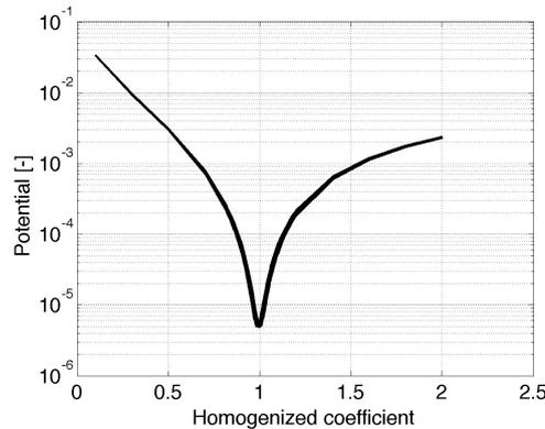
Figure 6. Value of the potential  $\int_{\underline{D}} |1 - \partial_x \underline{u}_\epsilon| dx$  as a function of the coefficient of the tentative homogenized medium, for  $\epsilon = 10$ , and for  $n = 10$  different ensembles of  $10^4$  realizations of the random medium.
