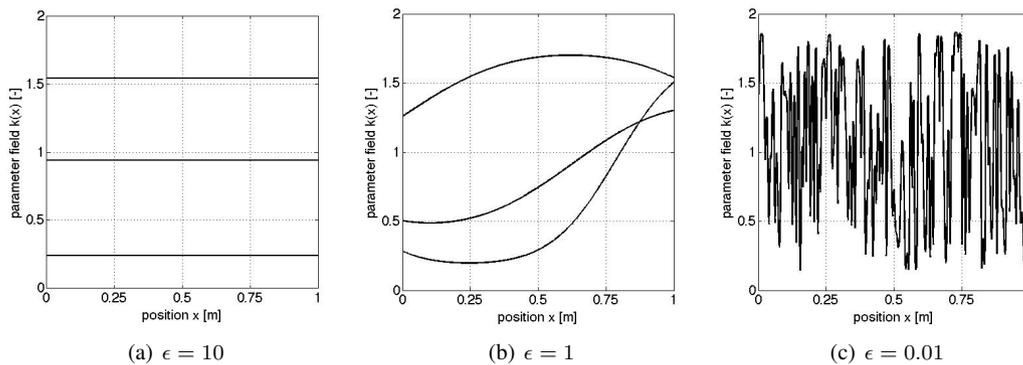
Figure 7. Three realizations of the random field  $\mathbf{k}_\epsilon(x)$  for three correlation lengths ((a)  $\epsilon = \ell_c/L = 0.01$ , (b)  $\epsilon = 1$ , and (c)  $\epsilon = 10$ ). For  $\epsilon = 0.01$ , only one realization is plotted for clarity.
