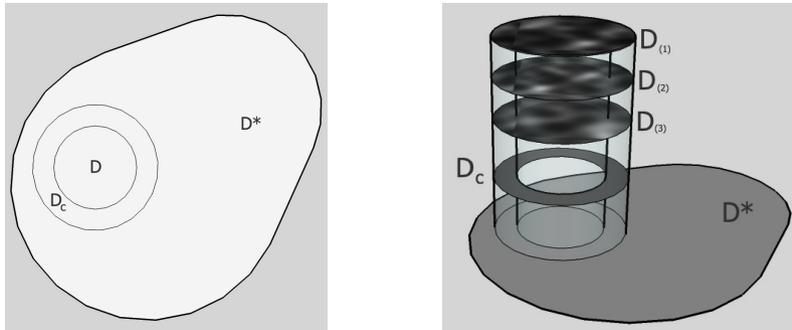
Figure 2. Section (left) and perspective view (right) of a 2D Arlequin problem where an effective model, defined over domain  $\underline{D}$ , and several realizations of a random model, defined over  $D$ , are coupled through a coupling domain  $D_c$ . On the overlap outside of  $D_c$ :  $(D \cap \underline{D}) \setminus D_c$ , both models are defined but behave independently.
