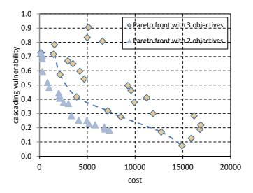
Figure 5. Comparison of the Pareto dominance fronts between three and two objectives optimization
