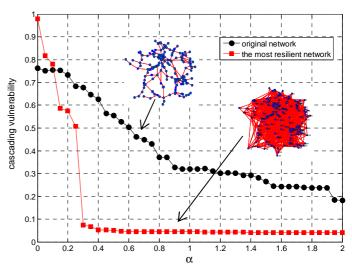
Figure 4. Comparison of the cascading vulnerability between the original and the most resilient networks under different network tolerance
