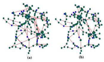
Figure 6. Comparison of the topology of the original network and a network corresponding to one of the 2-objectives optimization solutions (310.6, 0.59); square nodes are generators and circle nodes are distributors.
