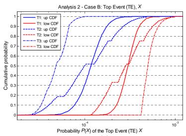
Figure 9. Upper and lower CDFs  $\overline{F}^{P(X)}$  and  $\underline{F}^{P(X)}$  obtained for P(X) under the assumptions of independence (solid lines), perfect (dashed lines) and unknown (dot-dashed lines) epistemic dependence (Configurations T1-T3 of Analysis 2 in Table III), with reference to Case B
