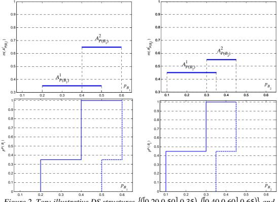
Figure 2. Top: illustrative DS structures  $\{([0.20,0.50],0.35), ([0.40,0.60],0.65)\}$  and  $\{([0.10,0.35],0.45), ([0.30,0.45],0.55)\}$  for  $P(B_1)$  (left) and  $P(B_2)$  (right), respectively. Bottom: upper (solid line) and lower (dashed line) CDFs,  $\overline{F}^{P(B_1)}$ ,  $\overline{F}^{P(B_2)}$ ,  $\overline{F}^{P(B_1)}$  and  $\overline{F}^{P(B_2)}$ , respectively, corresponding to the illustrative DS structures described above
