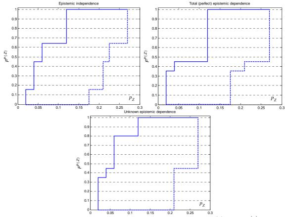
Figure 3. Upper (solid lines) and lower (dashed lines) CDFs,  $\overline{F}^{P(Z)}$  and  $\underline{F}^{P(Z)}$ , of the probability (chance) P(Z) of the conjunction of two (objectively) independent events  $B_1$  and  $B_2$  with probabilities (chances)  $P(B_1)$  and  $P(B_2)$  distributed as in Figure 2, under the assumptions of independence (top left), total (top right) and unknown (bottom) epistemic dependence
