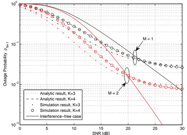
Fig. 3. The outage probability curves versus the transmit SNR in a wireless multihop network with  $N = 5$  for non-cooperative ( $M = 1$ ) and cooperative ( $M = 2$ ) cases, different spatial reuse factors, and  $R = \frac{1}{2}$  bits/sec/Hz.
