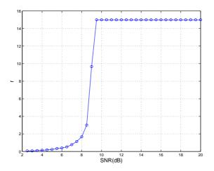
Figure 3: Required r versus SNR for BER  $\leq 10^{-2}$ .
