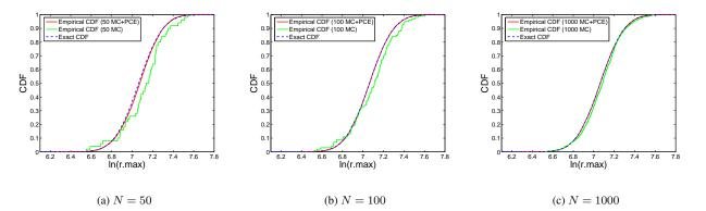
analytically (dashed blue line), for N = 50, 100, 1000(subfigures (a), (b) and (c) respectively). Even the meta-model built out of 50 samples reproduces the response variability quite closely; for N = 100 the approximation is very accurate without showing significant gains with respect to N = 1000. Therefore, a reasonable value for the parameter N is N = 100: this choice seems to balance the most the precision in the CDF estimate and the corresponding computational cost.
