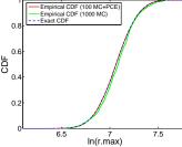
Figure 5: Comparison of the meta-model CDF obtained with an experimental design of size N = 100(red line) with the exact CDF (dashed blue line) and with the empirical CDF obtained with 1000 standard MC-simulations (green line)
