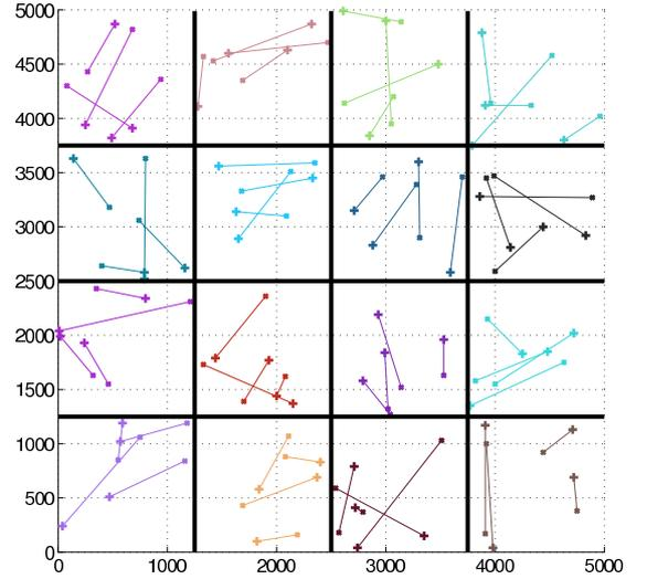
Fig. 3. A 5 km  $\times$  5 km square field divided into  $K = 16$  cells. Nodes are positioned randomly inside each cells.
