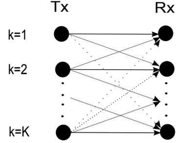
Fig. 1. Simplified system model: symmetric parallel interference channel.
