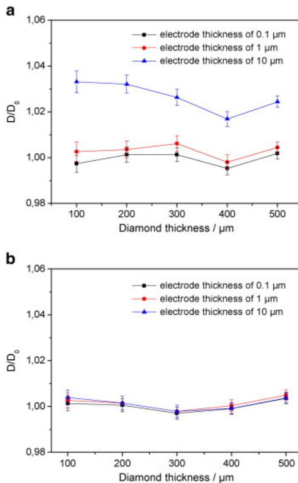
**Fig. 3.** Study of the influence of 1 mm diameter electrodes on the absorbed dose in the diamond in regard to the ratio of the mean absorbed dose  $D$  in the diamond sensitive volume in presence of electrodes to the mean absorbed dose  $D_0$  without electrodes, for a 6 MV photon beam and a  $2\text{ cm} \times 2\text{ cm}$  field size. a: Results for gold electrode on one diamond face and nickel electrode on the second face. b: Results for aluminum electrodes on both sides of the diamond.
