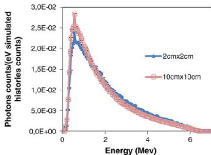
**Fig. 1.** Energy spectra of photons calculated in air, at 90 cm from the target of a Saturne 43 linac, for 6 MV photon beams, for a  $2 \times 2 \text{ cm}^2$  and a  $10 \times 10 \text{ cm}^2$  field. Spectra resolution: 50 keV. Spectra are normalized to the total number of photons recorded in each PSF.
