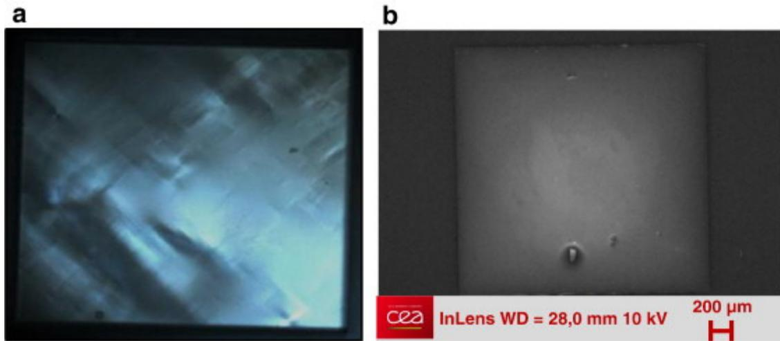
**Fig. 5.** Birefringence (a) and SEM images (b) of Element Six synthetic single crystal diamond selected for diamond dosimeter.
