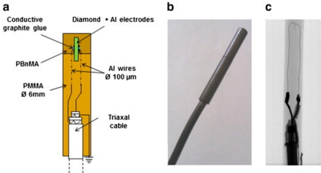
**Fig. 4. a.** Schema of water-equivalent SCDDo.
