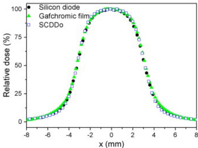
**Fig. 10.** Cross-line dose profiles measured with SCDDo, the PTW diode 60017 and Gafchromic films, for a 6MV photon beam and a  $6 \times 6 \text{ mm}^2$  beam size, with a Varian Clinac 2100 C linac and a  $\mu\text{MLC m3}$ . Depth of measurements: 10 cm in water. SSD of 100 cm.
