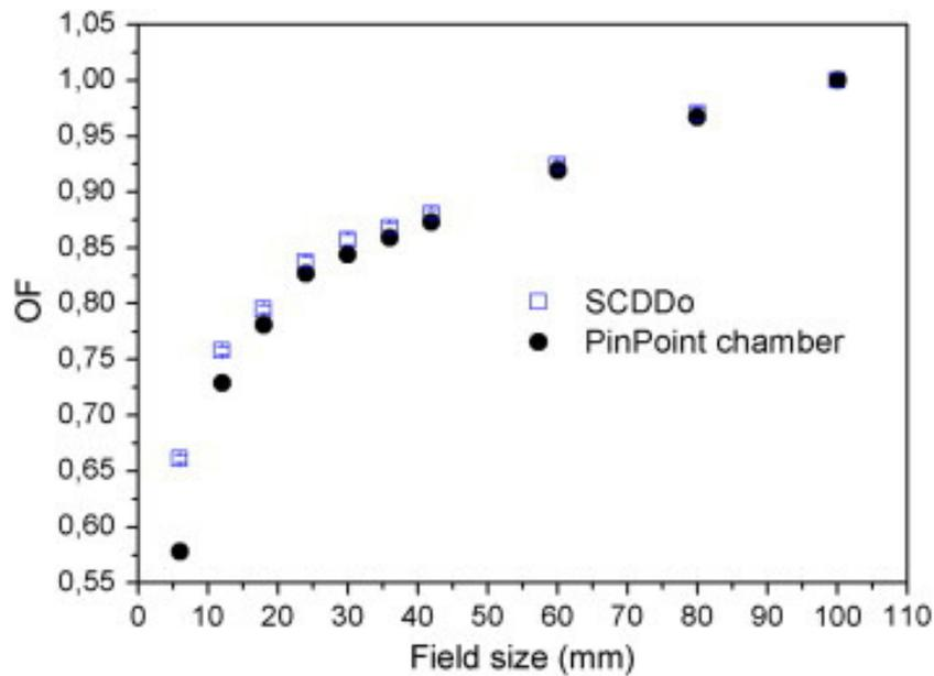
**Fig. 11.** Output factors measured with SCDDo (square data points and error bars) and a PinPoint chamber (circle data points), for 6MV photon beam, with a Varian Clinac 2100 C linac and a  $\mu$ MLC m3. Depth of measurements: 10 cm in water. SSD of 100 cm.
