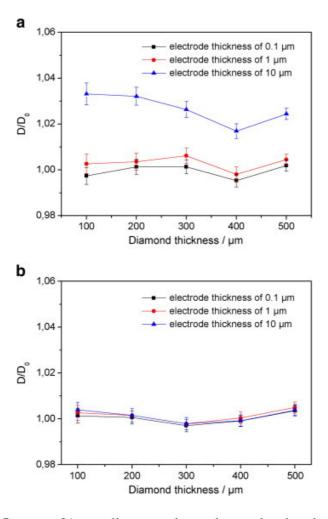
**Fig. 3**. Study of the influence of 1 mm diameter electrodes on the absorbed dose in the diamond in regard to the ratio of the mean absorbed dose D in the diamond sensitive volume in presence of electrodes to the mean absorbed dose  $D_0$  without electrodes, for a 6 MV photon beam and a 2 cm  $\times$  2 cm field size. a: Results for gold electrode on one diamond face and nickel electrode on the second face. b: Results for aluminum electrodes on both sides of the diamond.
