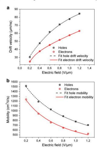
Fig. 7. Drift velocity (a) and mobility (b) values as a function of applied electric field.
