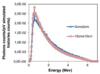
**Fig. 1**. Energy spectra of photons calculated in air, at 90 cm from the target of a Saturne 43 linac, for 6 MV photon beams, for a  $2 \times 2$  cm<sup>2</sup> and a  $10 \times 10$  cm<sup>2</sup> field. Spectra resolution: 50 keV. Spectra are normalized to the total number of photons recorded in each PSF.
