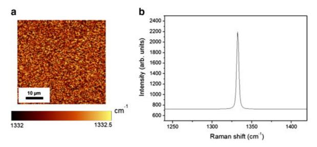
**Fig. 6. a**: Diamond peak position measured with confocal micro-Raman spectroscopy on a surface of  $50 \ \mu m \times 50 \ \mu m$ .
