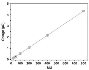
**Fig. 8.** Dose dependence of SCDDo response. Error bars are less than the height of data points ( $\square$ ). Linear fit is plotted with solid line.
