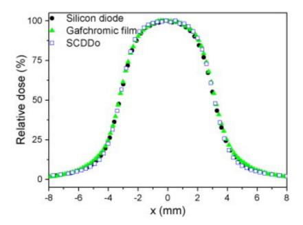
**Fig. 10**. Cross-line dose profiles measured with SCDDo, the PTW diode 60017 and Gafchromic films, for a 6MV photon beam and a  $6 \times 6$  mm<sup>2</sup> beam size, with a Varian Clinac 2100 C linac and a  $\mu$ MLC m3. Depth of measurements: 10 cm in water. SSD of 100 cm.
