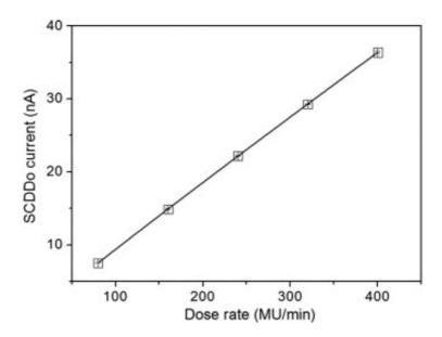
Fig. 9. Dose rate dependence of SCDDo response. Error bars are less than the height of data points  $(\Box)$ . Fowler's equation fit is plotted with solid line.
