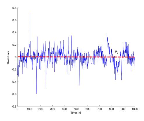
Fig. 8. Residuals: difference between measurements and reconstructions of Fig. 7.
