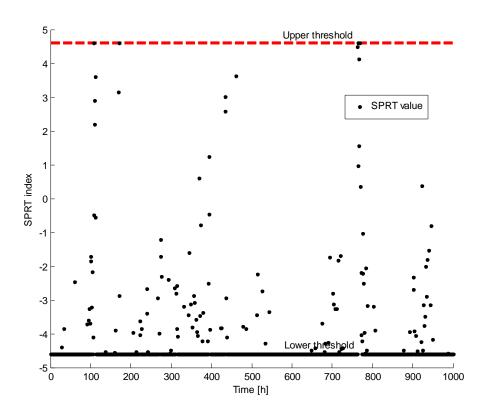
Fig. 9. Outcomes of the SPRT for the signals reconstructed in Fig. 7.
