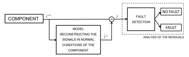
Fig. 1. Condition monitoring scheme for fault detection.
