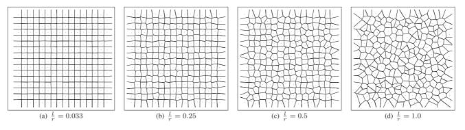
Fig. 3. Impact of the ratio  $\frac{l}{r}$  on the Voronoï cells.
