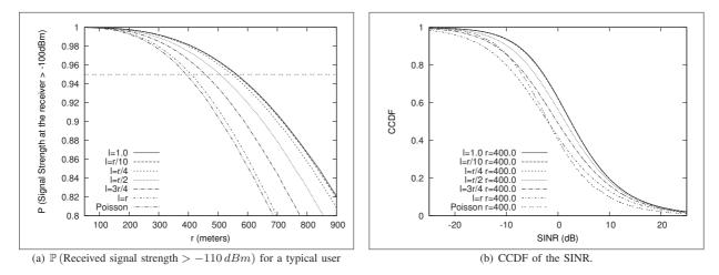
Fig. 4. CCDF of SINR and received signal strength
