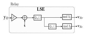
Fig. 3: Layered Lattice encoding at the relay
