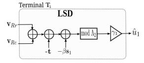
Fig. 4: Lattice source decoding at the Terminal 1
