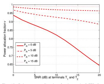
Fig. 10: Relay power allocation fraction  $\nu$  in LCF2 for different fixed relay transmit power  $P_R$  and equal SNR =  $\frac{P_1}{\sigma_R^2} = \frac{P_2}{\sigma_R^2}$  at both terminals,  $|h_1|^2 = 4$  and  $|h_2|^2 = 0.5$ .
