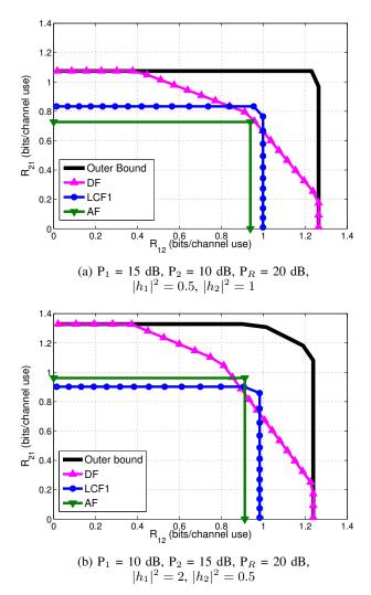
Fig. 5: Achievable rate regions and the outer bound capacity of the Gaussian TWRC. In the left,  $T_1$  has the best transmit power and the worst channel. In the right,  $T_2$  has the best transmit power and the worst channel.
