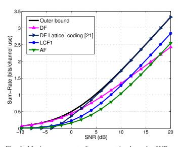
Fig. 6: Maximum sum-rate for symmetric channels:  $SNR = SNR_{1R} = SNR_{R1} = SNR_{2R} = SNR_{R2}$ . LCF1 outperforms AF and DF for SNR > 11 dB
