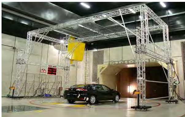
Figure 7: Acoustic imaging on the vehicle surface in Wind tunnel S2A.
