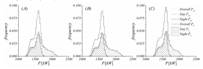
Figure 10. Total available  $P_{av}$  and used  $P_u$  power for configurations:  $\Xi_3^{DG}$  (A),  $\Xi_I^{DG}$  (B) and  $\Xi_2^{DG}$  (C)
