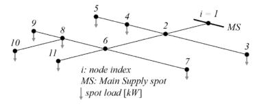
Table 3 contains the technical characteristics of the different types of feeders considered: specifically, the indexes of the pairs of nodes that are connected by each feeder of the network, their length, reactance *X* and their ampacity *Amp*.
