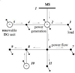
Figure 1. Example of a renewable DG-integrated network configuration
