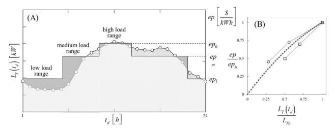
Figure 3. Example of load ranges definition for a generic daily load profile (A) and correlation energy price-total load (B) [5, 12, 13]
