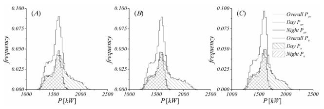
Figure 10. Total available  $P_{av}$  and used  $P_u$  power for configurations:  $\Xi_3^{DG}$  (A),  $\Xi_1^{DG}$  (B) and  $\Xi_2^{DG}$  (C)
