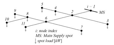
Figure 5. Radial 11-nodes distribution network
