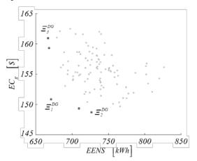
Figure 8. Pareto Front resulting from the MOO concerning the simultaneous minimization of EENS and EC<sub>g</sub> [11]
