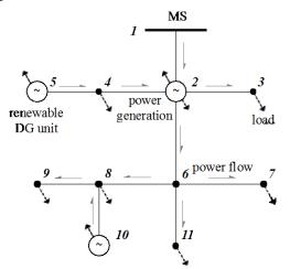
Figure 1. Example of a renewable DG-integrated network configuration
