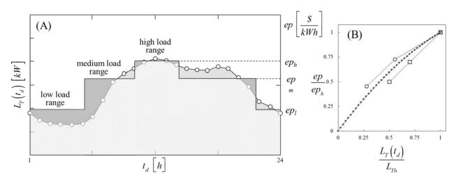
Figure 3. Example of load ranges definition for a generic daily load profile (A) and correlation energy price-total load (B) [5, 12, 13]
