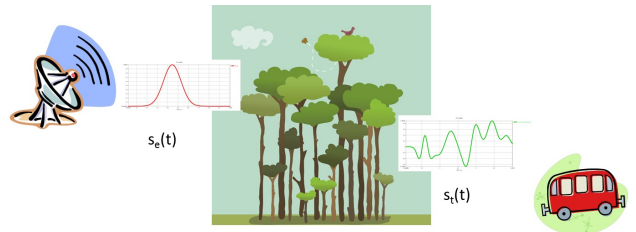
Fig. 1. A radar emits the signal s_e(t) which the forest modifies to s_t(t) before it reaches the target.
