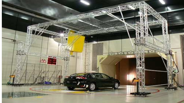
Figure 4: Acoustic imaging on the vehicle surface in Wind tunnel S2A.
