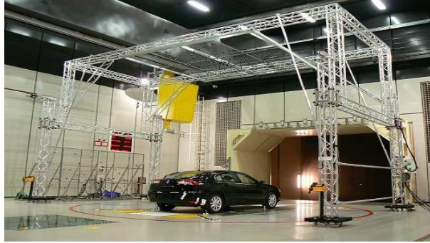
Figure 4: Acoustic imaging on the vehicle surface in Wind tunnel S2A.
