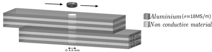
**Figure 10.** Cylindrical through-wall hole in two multi-layer slabs
