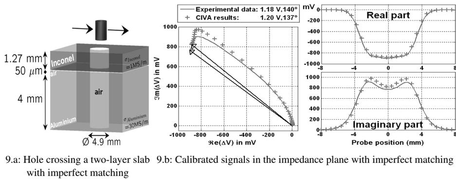
**Figure 9.** Cylindrical through-wall hole in a two-layer slab (— experimental data, +++ CIVA results)
