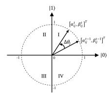
Figure 1. Polar plot of the rotation gate for updating one Q-bit
