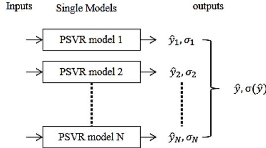
Figure 1. Paradigm of a typical ensemble method.
