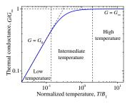
FIG. 2 (color online). Thermal conductance versus temperature for a nanowire with a single transmitted mode ( $N = N_0 = 1$ ).
