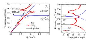
FIG. 3 (color online). (a) Dispersion relation and (b) propagation length as a function of the frequency, for the nanowires of SiC and SiO<sub>2</sub> surrounded by air ( $\varepsilon_2 = 1$ ).
