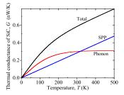
FIG. 5 (color online). Phonon and SPP components of the thermal conductance of SiC, as a function of temperature.
