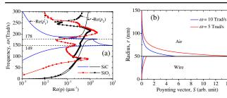
FIG. 4 (color online). (a) Frequency dependence of Re(p) inside and outside of the nanowires of SiC and SiO<sub>2</sub> surrounded by air. (b) Poynting vector for a nanowire of SiC with radius a = 50 nm, as a function of the radial coordinate.
