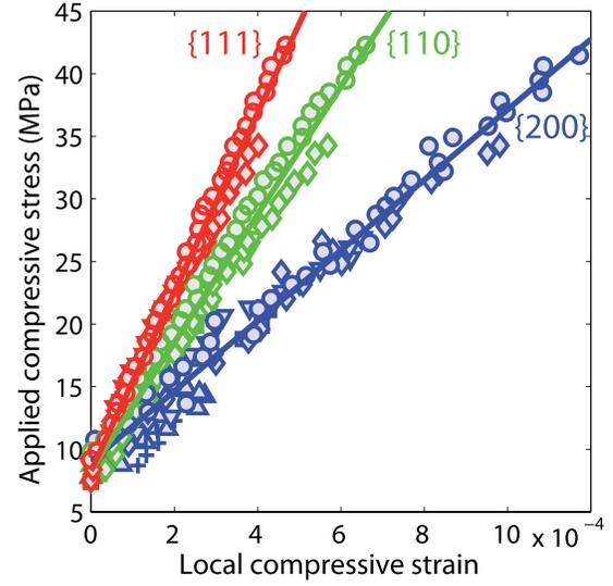
(a) Stress-strain curve for  $\psi=0$
