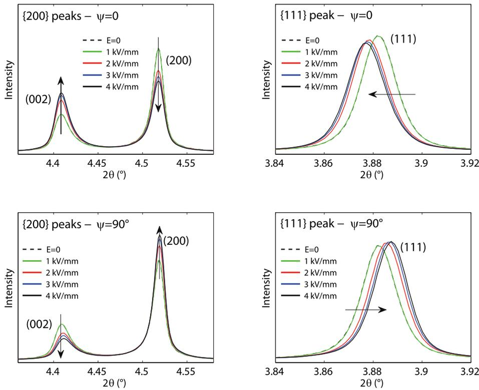
FIG. 20. Diffraction patterns for the first electric field loading (points A–B in Fig. 3): {111} and {200} peaks for  $\psi=0^\circ$  and  $\psi=90^\circ$ . The profiles are given for  $E=0, 1, 2, 3,$  and  $4$  kV/mm.
