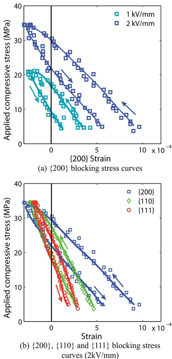
FIG. 18. Irreversibilities during the blocking force test. (a) {200} blocking stress curves obtained for  $\psi = 0$  at 1 and 2 kV/mm (a) and (b) {200}, {110}, and {111} blocking stress curves obtained for  $\psi = 0$  at 2 kV/mm. Experimental measurements (markers) and approximate evolution for eye guidance (lines). (a) {200} blocking stress curves and (b) {200}, {110}, and {111} blocking stress.
