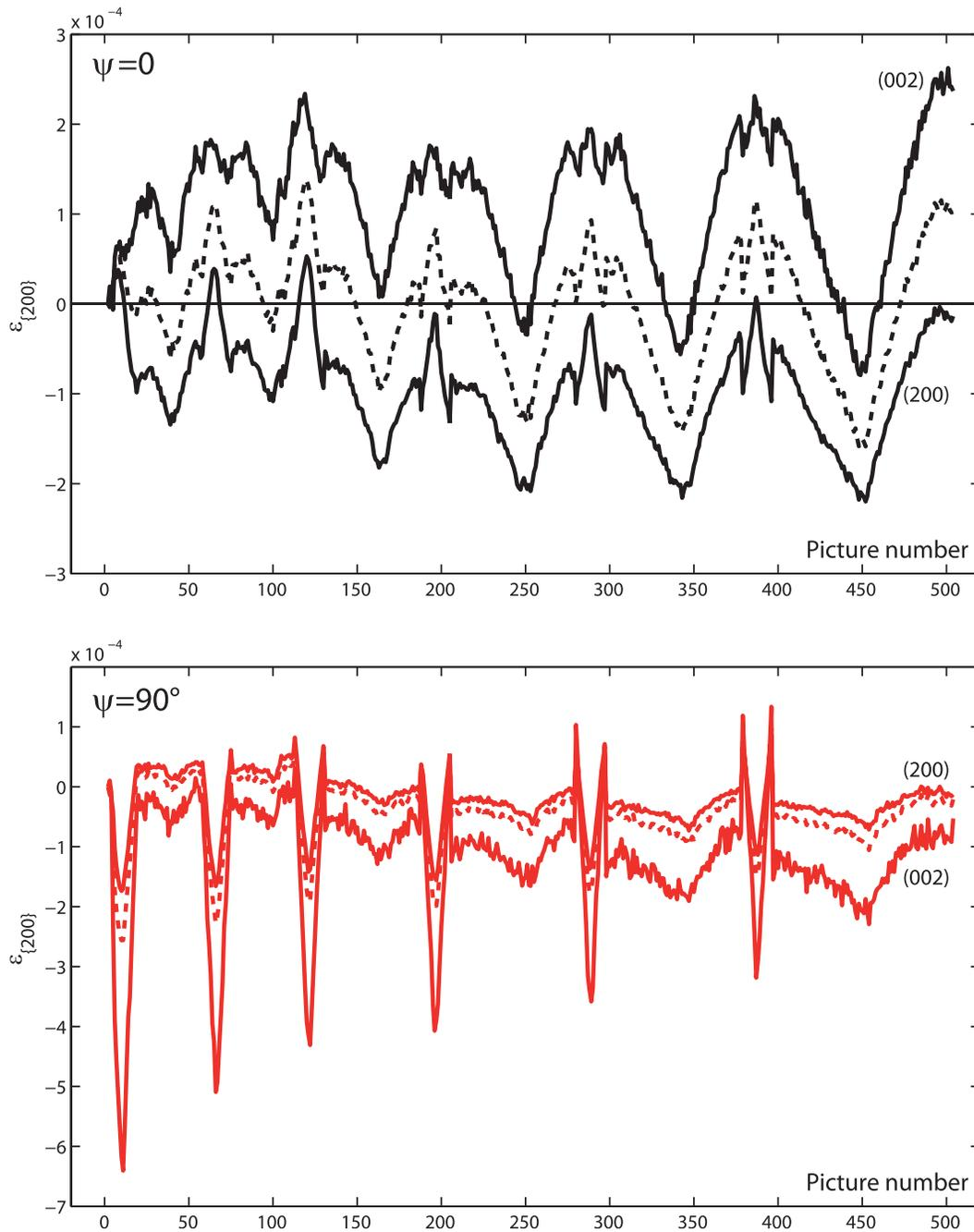
FIG. 16. Evolution of  $\varepsilon_{(002)}$  and  $\varepsilon_{(200)}$  during the *in-situ* blocking force test for the orientation  $\psi = 0^\circ$  (top) and  $\psi = 90^\circ$  (bottom). The dotted line is the weighted average of  $\varepsilon_{(002)}$  and  $\varepsilon_{(200)}$ . This graph illustrates the strain for this particular crystallographic orientation without incorporating the transformation strain.
