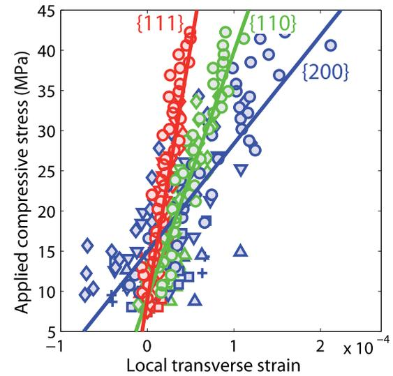
(b) Stress-strain curve for  $\psi=90^\circ$
