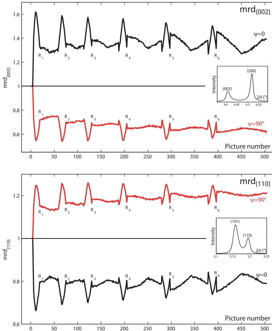
FIG. 4. Evolution of  $mrd_{002}$  and  $mrd_{110}$  during the *in-situ* experiment,  $\psi = 0$  and  $\psi = 90^\circ$ .  $mrd_{002}$  (respectively,  $mrd_{110}$ ) defines the relative intensities of  $\{200\}$  (respectively,  $\{110\}$ ) peaks and quantifies domain switching processes.
