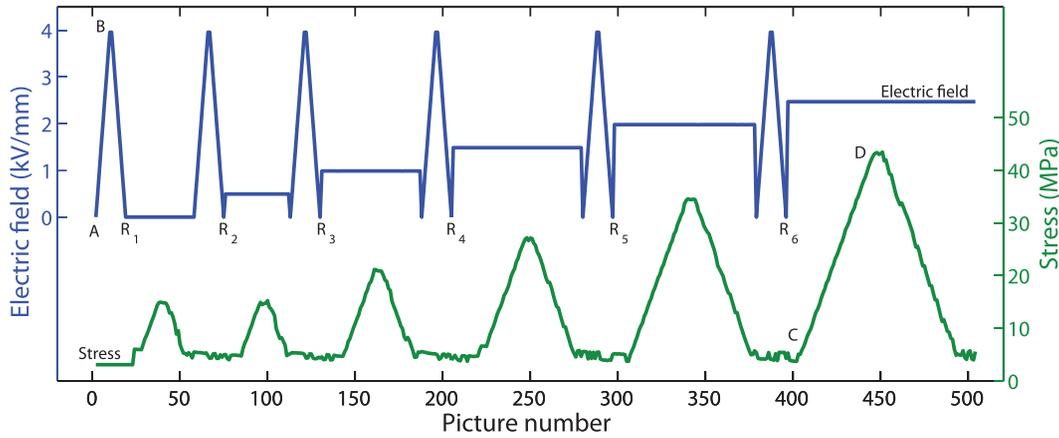
FIG. 3. External electromechanical loading during the *in-situ* experiment: electric field (top) and compressive stress (bottom).
