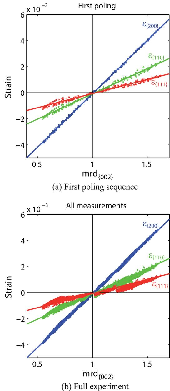
FIG. 15. Correlation between multiple of random distribution  $mrd_{002}$  and local strain for different crystallographic orientations. All orientations  $\psi$  are regrouped on the figure. (a) First poling sequence and (b) full experiment.
