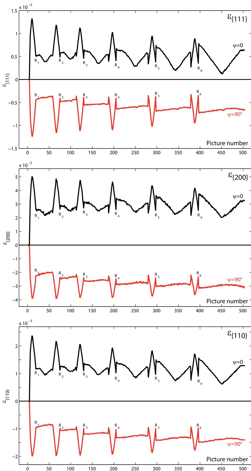
FIG. 5. Evolution of  $\varepsilon_{\{111\}}$ ,  $\varepsilon_{\{200\}}$ , and  $\varepsilon_{\{110\}}$  during the *in-situ* experiment,  $\psi = 0^\circ$  (top) and  $\psi = 90^\circ$  (bottom).
