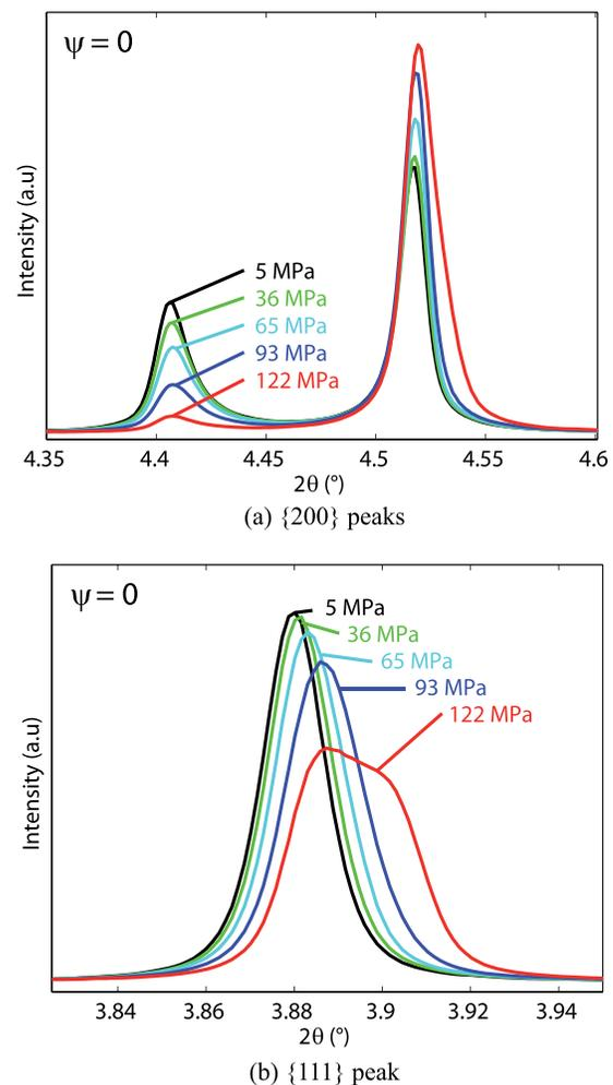
FIG. 19. Diffraction patterns for PZT51-49 under compressive stress from 36 to 122 MPa (no applied electric field) for  $\psi = 0$ . The pattern at 122 MPa reveals a phase change under stress for the material. (a) {200} peaks and (b) {111} peak.
