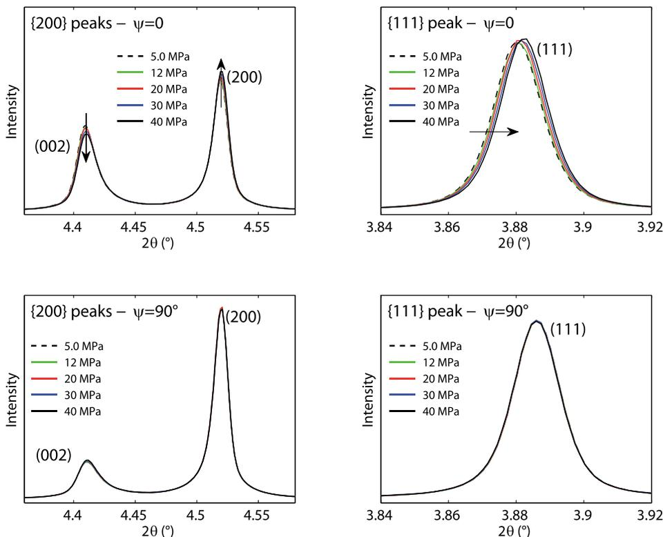
FIG. 21. Diffraction patterns for the last stress loading (points C–D in Fig. 3): {111} and {200} peaks for  $\psi=0^\circ$  and  $\psi=90^\circ$ . The patterns show very little domain switching under stress. The profiles are given for  $\sigma=5.0, 12, 20, 30,$  and  $40$  MPa.
