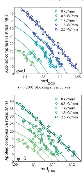
FIG. 13. Blocking stress curves showing domain switching during the blocking force test. Results obtained for  $\psi=0$  at several levels of electric field. Experimental measurements (markers) and trend lines to guide the eye. (a) {200} blocking stress curves and (b) {110} blocking stress curves.
