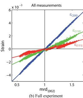
FIG. 15. Correlation between multiple of random distribution  $\mathrm{mrd}_{002}$  and local strain for different crystallographic orientations. All orientations  $\psi$  are regrouped on the figure. (a) First poling sequence and (b) full experiment.
