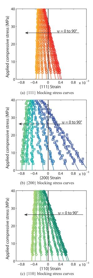
FIG. 7. Analysis of diffraction profiles: blocking stress curves obtained for  $\psi=0^{\circ}-90^{\circ}$  ( $10^{\circ}$  steps) for an applied electric field of 2.5 kV/mm. Experimental measurements (markers) and corresponding linear fitting (lines). (a) {111} blocking stress curves, (b) {200} blocking stress curves, and (c) {110} blocking stress curves.
