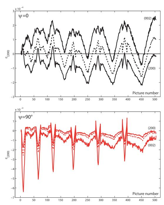
FIG. 16. Evolution of  $\varepsilon_{(002)}$  and  $\varepsilon_{(200)}$  during the *in-situ* blocking force test for the orientation  $\psi = 0^{\circ}$  (top) and  $\psi = 90^{\circ}$  (bottom). The dotted line is the weighted average of  $\varepsilon_{(002)}$  and  $\varepsilon_{(200)}$ . This graph illustrates the strain for this particular crystallographic orientation without incorporating the transformation strain.
