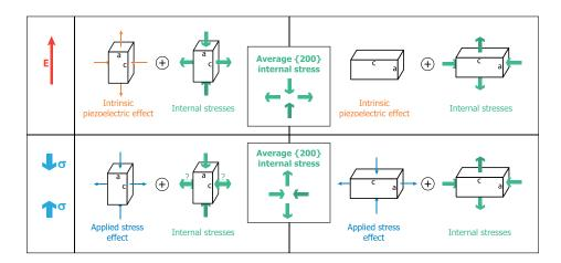
FIG. 17. Schematic view of the effect of an applied load (electric field or stress) for 200 oriented grain as a function of the local polarisation direction. The contributions due to the piezoelectric effect, internal stresses resulting from domain switching and the elastic effect due to the applied stress are separated.
