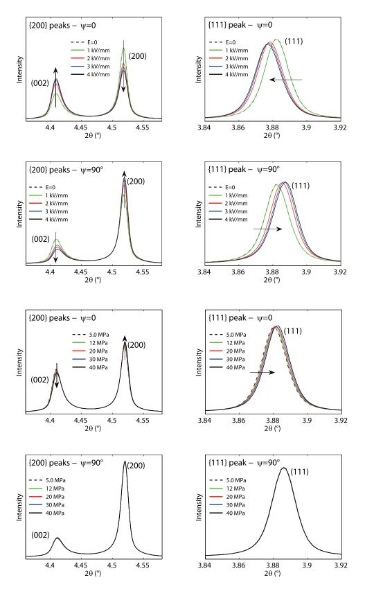
FIG. 20. Diffraction patterns for the first electric field loading (points A–B in Fig. 3): {111} and {200} peaks for  $\psi=0^{\circ}$  and  $\psi=90^{\circ}$ . The profiles are given for E=0,1,2,3, and 4 kV/mm.
