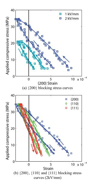
FIG. 18. Irreversibilities during the blocking force test. (a) {200} blocking stress curves obtained for  $\psi=0$  at 1 and 2 kV/mm (a) and (b) {200}, {110}, and {111} blocking stress curves obtained for  $\psi=0$  at 2 kV/mm. Experimental measurements (markers) and approximate evolution for eye guidance (lines). (a) {200} blocking stress curves and (b) {200}, {110}, and {111} blocking stress.
