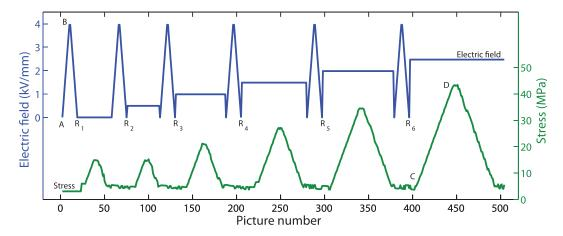
FIG. 3. External electromechanical loading during the in-situ experiment: electric field (top) and compressive stress (bottom).
