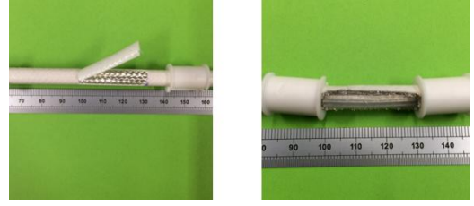
Fig. 5. Shield damage at 8.4 m on a 25 m coaxial cable EN 0406 WD, with different length (i.e., 1, 2, 3 cm).
