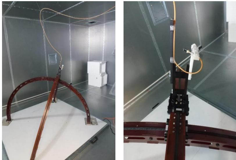
**Fig. 1 :** The robot optimized to weakly perturbate a reverberation chamber in the GHz range. On the right, a detail showing the electro-optic probe.
