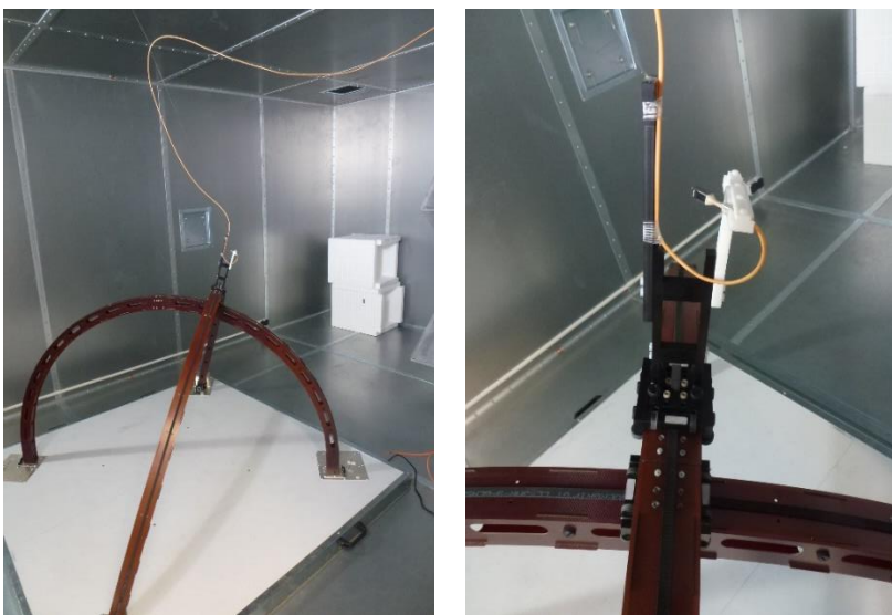
Fig. 1 : The robot optimized to weakly perturbate a reverberation chamber in the GHz range. On the right, a detail showing the electro-optic probe.
