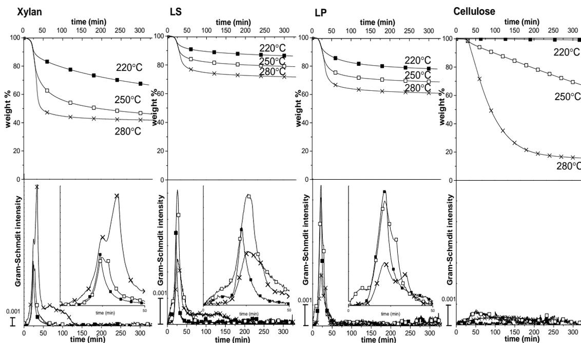
**Fig. 1.** Mass loss and Gram-Schmidt curves of torrefied samples. The upper graphs represent mass loss, and the lower graphs indicate G-S intensity (an intensity of 0.001 scale bar is provided; partial magnified graphs are embedded). The line with solid squares is for torrefaction at 220 °C; the line with hollow squares is for torrefaction at 250 °C; the line with crosses is for torrefaction at 280 °C.
