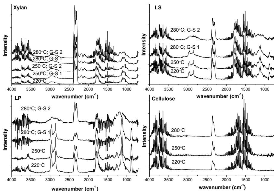
**Fig. 2b.** IR spectra obtained at the maximum evolution rate of corresponding 3D spectrograms of Fig. 2a. G-S 1 represents the spectrum from the first G-S peak, and G-S 2 represents the spectrum from the second G-S peak.
