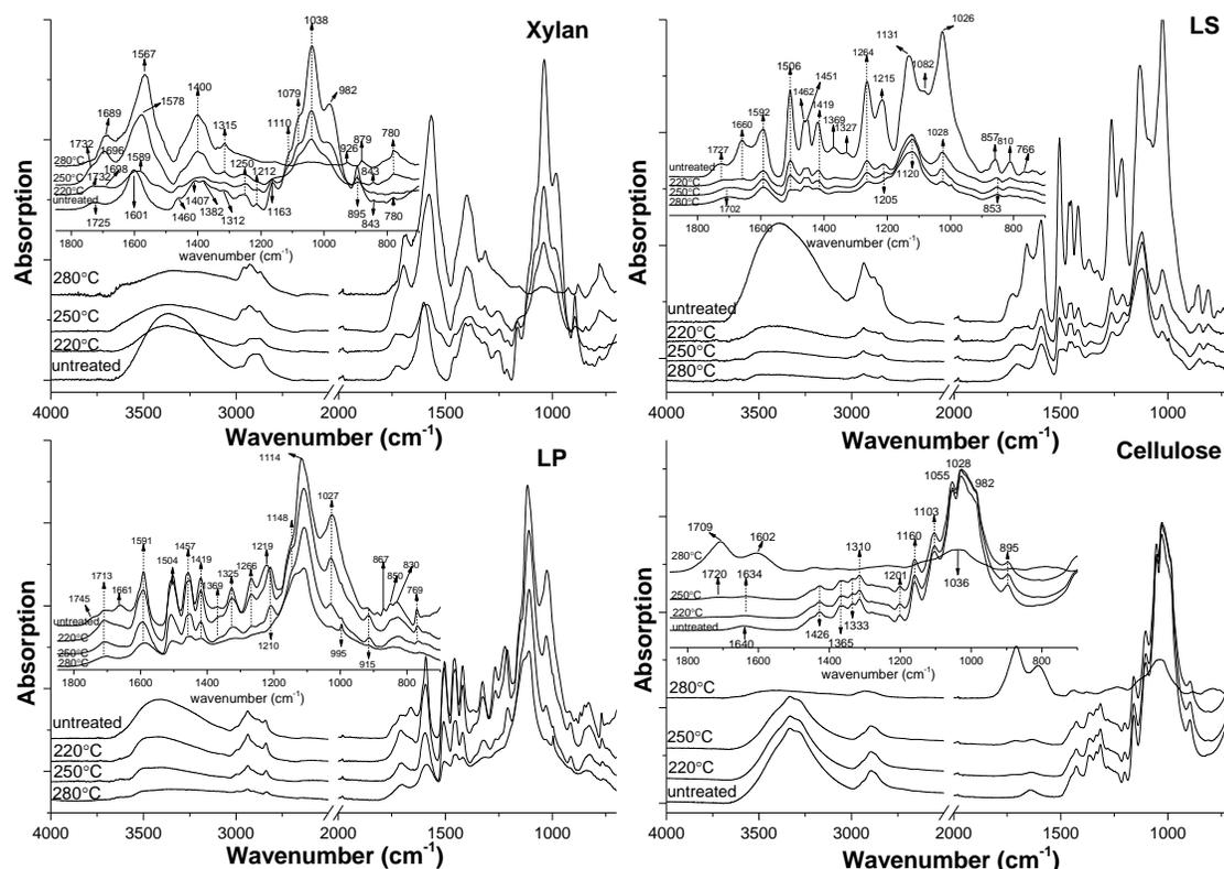
Fig. 3. FTIR-ATR spectra of torrefied and untreated samples
