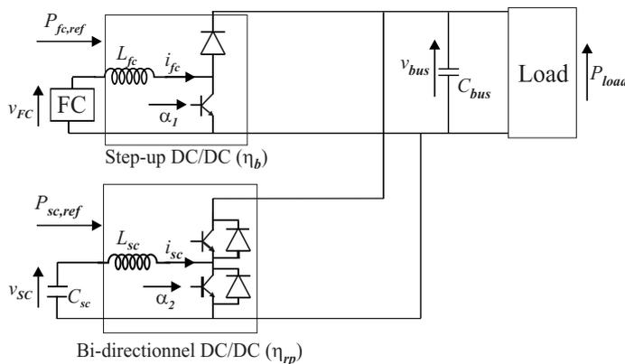
Fig. 1. Fuel cell/supercapacitor architecture
