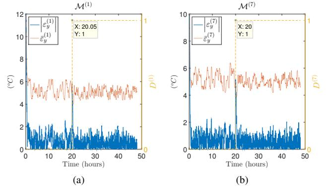
Fig. 2. Residuals  $\varepsilon^{(1)}$ ,  $\varepsilon^{(7)}$  (blue solid line), adaptive thresholds  $\bar{\varepsilon}^{(1)}$ ,  $\bar{\varepsilon}^{(7)}$  (red dotted line) and detection signals  $D^{(1)}$ ,  $D^{(7)}$  (yellow dashed line) of the monitoring agents  $\mathcal{M}^{(1)}$ ,  $\mathcal{M}^{(7)}$
