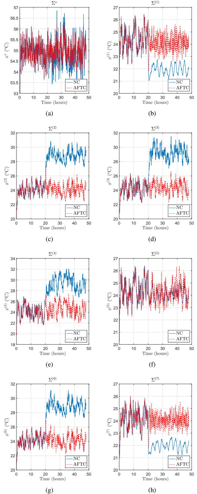
Fig. 3. HVAC system temperature response in multiple simultaneous bias sensor fault scenario in sensors  $S^{(1)}$ ,  $S^{(7)}$ : controlled by the nominal control (NC) scheme (blue solid line), controlled by the adaptive fault-tolerant control (AFTC) scheme (red dashed line)
