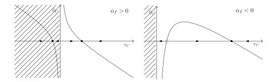
Figure 3: Plot of  $\dot{v}_C$  versus  $v_C$  for the cases of (a)  $\alpha_I > 0$  and (b)  $\alpha_I < 0$ . The arrows in the horizontal axis indicate the direction of the flow of the zero dynamics.
