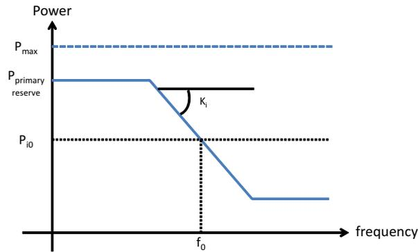
**Figure 1** Power-frequency curve for a traditional unit
