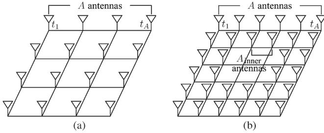
Fig. 1. Examples of the transmit antenna array. (a)  $N_t = 16$ . (b)  $N_t = 32$ .
