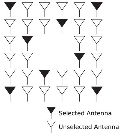
Fig. 3. RCP for selecting 8 out of 32 antennas.
